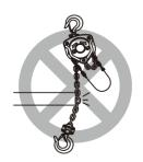
NEVER run the load chain over a sharp edge
