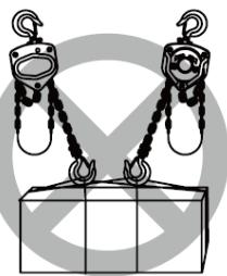
NEVER use two or more hoists together to lift beyond a hoist's rated capacity.
