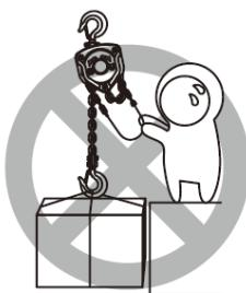
NEVER lift a load heavier than a hoist's rated capacity.
