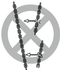
NEVER use a twisted, kinked, damaged or stretched load chain
