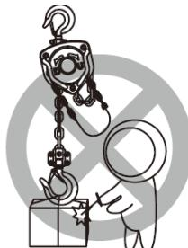
NEVER weld or cut a load suspended by a chain block
