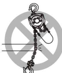
NEVER run the load chain over a sharp edge
