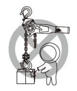
NEVER weld or cut a load suspended by a ratchet puller
