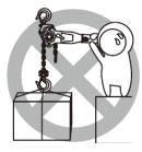
NEVER lift a load heavier than a puller's rated capacity.
