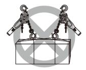
NEVER use two or more pullers together to lift beyond a puller's rated capacity.
