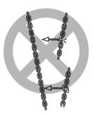
NEVER use a twisted, kinked, damaged or stretched load chain.
