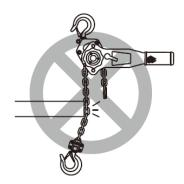
NEVER run the load chain over a sharp edge
